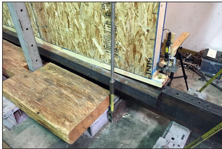
Figure 10. Typical uplift for the ASTM E72 racking test.
