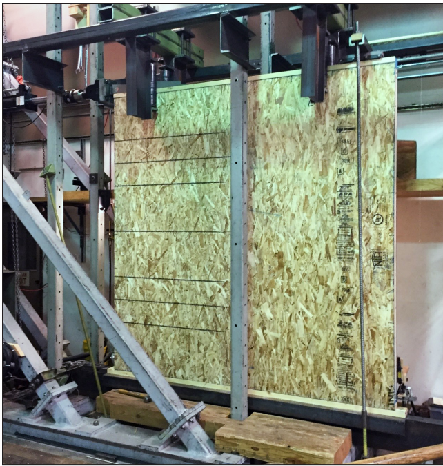
Figure 6. ASTM E72 monotonic test setup.
