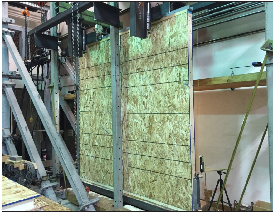
Figure 8. CUREE cyclic test setup.
