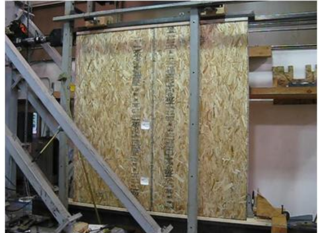
Figure E2. Wall loaded in test rack for cyclic test, note cut-outs in OSB for electrical boxes.
