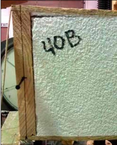
Figure 14. Short-term bending, typical failure mode (OSB bending) of foam flush detail (top) and typical failure mode (tearing of EPS foam) of 2x end block detail (bottom) (APA–The Engineered Wood Association).
