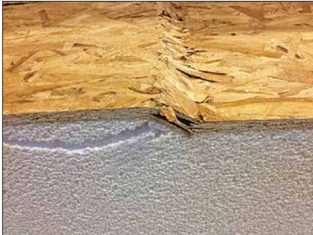
Figure 13. Compression failure (FPL).
