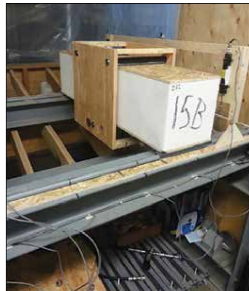
Figure 7. Creep test setup (APA-The Engineered Wood Association).
