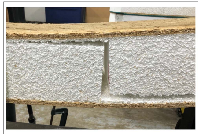
Figure 4.—Shear failure mode in exemplar 16.5-cm (6.5-in.)-class beam. All beams in this depth class failed by this same mode.
