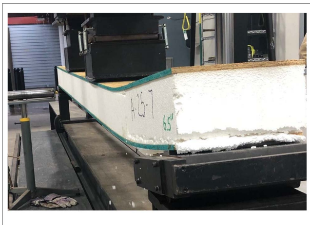
Figure 3.—Photograph of 16.5-cm (6.5-in.)-class beam in the testing machine at the time of failure.
