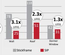
Source: BASF Time-Motion Study, 2 x 6 stud at 16" oc vs. 6.5" SIP panel
