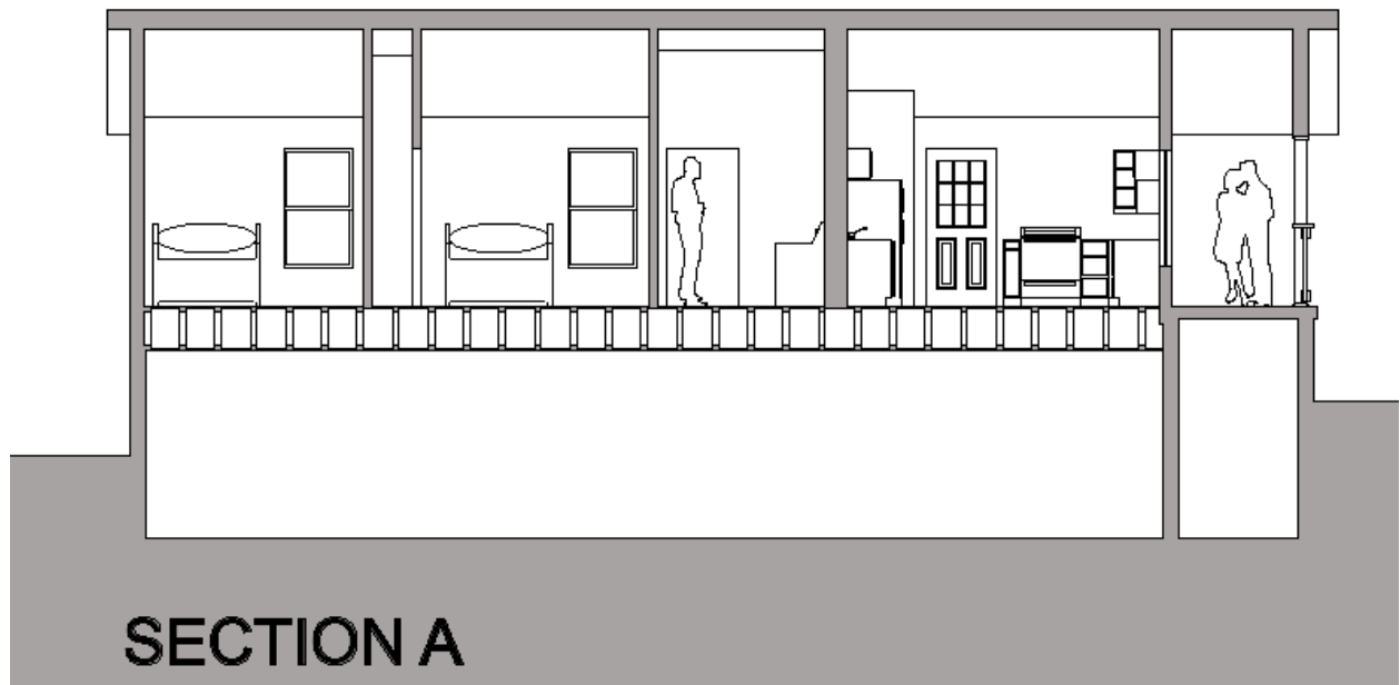
Figure 12. Longitudinal section through ZEH5, location marked on the floor plan in Figure 4.
